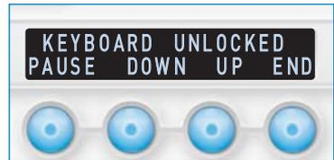
**NOTE:** The Button Lock will be disabled when the Reset button is pressed or when turning the power off.
