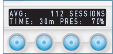
4. Press any button to return to the Information Menu. If a button is not pressed within 30 seconds, the display will return to the Information Menu automatically. See the Reset Defaults section to clear the session count and average use information.
